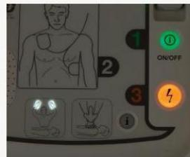
The device will announce whether or not a shock is advised. If shock is advised, there will be a continuous beep and the shock button will flash orange. Press the flashing orange shock button when prompted:
