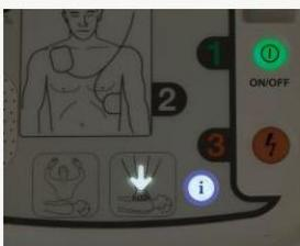
**If a shock has been delivered**, the i button will flash blue and can be pressed for CPR voice prompt.
